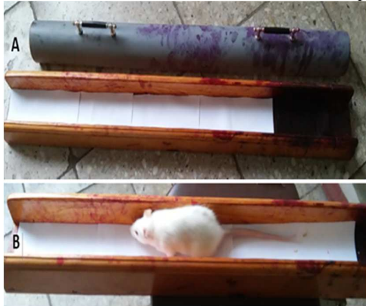
Fig. 2. Walking Track device during obtaining rat footprints. A – general view; B – view of walking animal without half cut plastic pipe.
