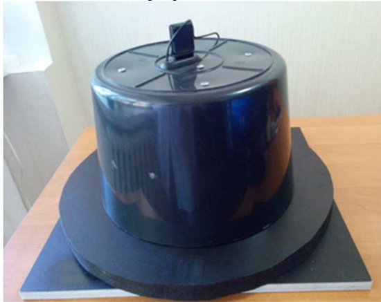
Figure 3. Outer appearance of a photobox for taking pictures of masticatory test fragments
